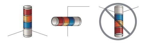
$\divideontimes$  For products with a protection rating of less than IPX4, please install it vertically.
